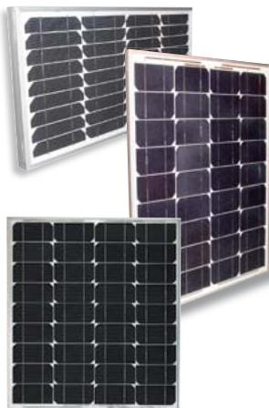
Istar Solar® photovoltaic modules **IS30P, IS40P and IS50P** with powers of **30Wp, 40Wp and 50Wp**, are composed of 36 high efficiency monocrystalline cells. These modules have a nominal voltage of 12V and are designed for any kind of stand alone system.
