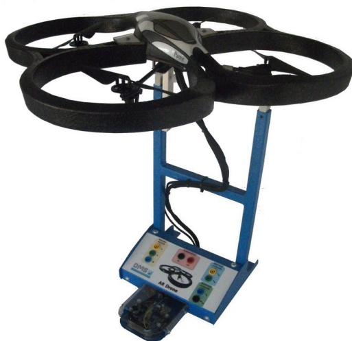
Fig. 109: Maquette AR.Drone en position "Orienter"
